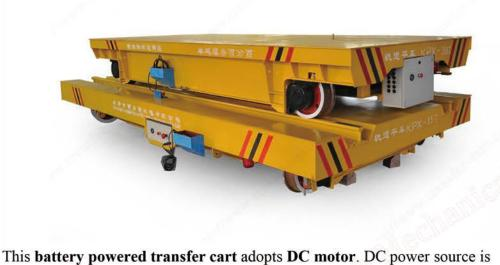
the transfer cart to run. DC motor has the advantages of stable start, large start torque, suitable for repeatedly start and saving energy.
